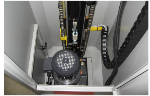
Inside the tower, dual ANSI chain and cable track are used for smooth carriage movement. The Sentry uses no-maintenance AC motors with VFD.
