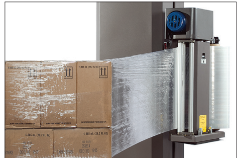
The film carriage prestretches film 200% prior to wrapping. This reduces material costs and strengthens the film for a tighter and more secure wrap. The machine E-stops if carriage detects an obstacle.
