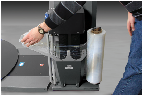
Loading film is fast and easy: open the hinged door, pull the film tail through, and close the door. Power is disconnected when the door is opened.
